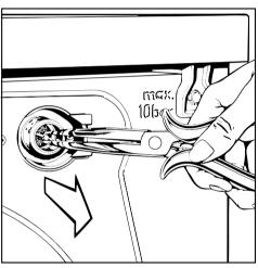
■ Using needle nose pliers, withdraw the plastic filter by pulling on the bar (see illustration). Rinse under water to clean, and then replace.
